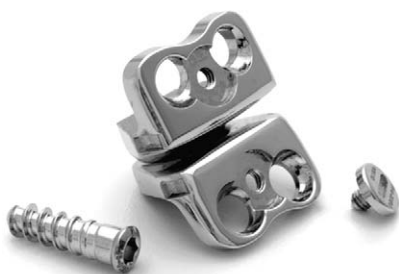
Fig. 1. The Prestige ST total joint replacement device consists of two articulating components that are attached to the adjacent vertebral bodies by four bone screws. A locking cap screw prevents back-out of the bone screws.
